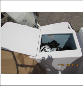
NO Gasket Installed on Lid of LPG Locker
